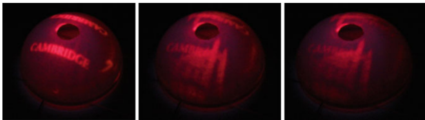
Fig. 1.24 Experimental images from the LC/antenna device. Left , 0 V applied ( vertical ). Centre , 0.44 \text{ V } \mu\text{m}^{-1} applied ( 45^\circ ). Right , 0.65 \text{ V } \mu\text{m}^{-1} applied ( horizontal )
